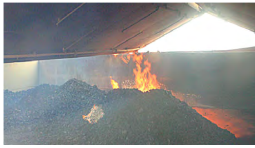
Cargo of coal on fire
